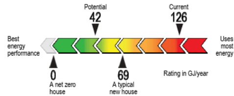
Figure 4. As part of the EnerGuide evaluation a renovation upgrade report is produced which recommends energy saving upgrades as well as this graphic displaying the current and potential energy performance of the building.
